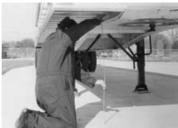
Figure 5. Measure the actual kingpin height
