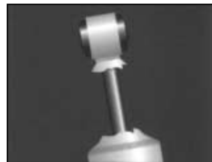
Broken dust tube
