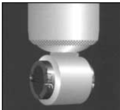
Broken upper or lower bushing These can be replaced very easily and are considered a regular maintenance item on a shock absorber.
